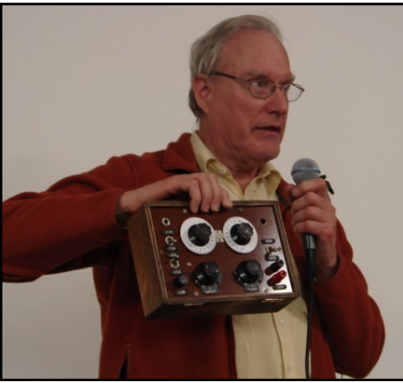
Nevell Greenough reproduced Al Klase's "Skywaves" crystal set. Built with toroid coils, Nevell says that the radio is a great performer using a 1N34A detector and won first place in the crystal set category of our last DX contest.
