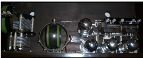
Tuska 305 "Superdyne" showing variometer supplying negative feedback.
