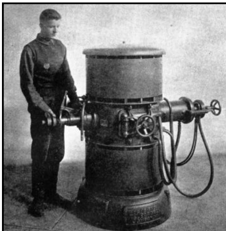
A production model Federal Telegraph arc transmitter. Although the size is not stated in the photo data, it is likely in the 30 kW range. (Courtesy of History San José)
