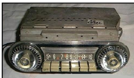
Stromberg-Carlson 85SE, AM push-button radio that appeared in the 1958 Edsel Ranger, Pacer, Corsair and Citation.
