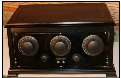
In 1924, the company offered a 3-dial, 5-tube (199s) "Super Parmak" TRF set.
