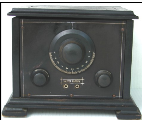
The high-end model 733, 1937 Parmak "Masterpiece" farm radio with 3 RF and 3 IF stages, two short wave bands, push-pull output and two speakers.
