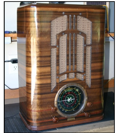
The high-end model 733, 1937 Parmak "Masterpiece" farm radio with 3 RF and 3 IF stages, two short wave bands, push-pull output and two speakers.
