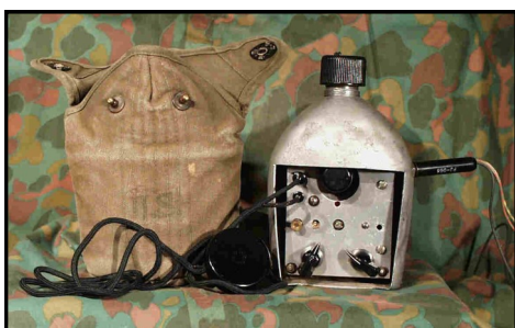
Al Klase's reproduction of a prisoner of war canteen radio used in the Philippines.
