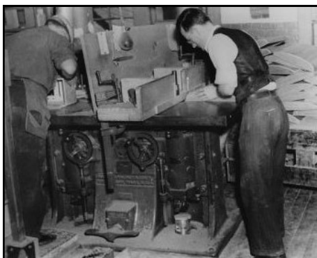
Using a double spindle sander in the Ingraham Case Shop in 1940.
