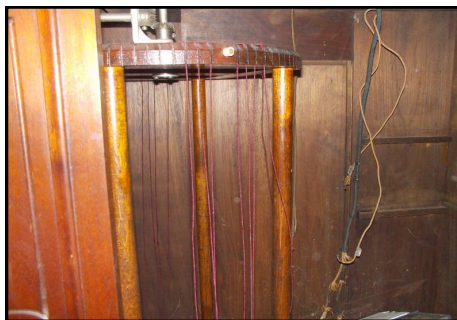
W-6-F base showing rotating antenna drum and gear mechanism. Two examples of this radio show this setup in their base, with one base also enclosing a battery eliminator.
