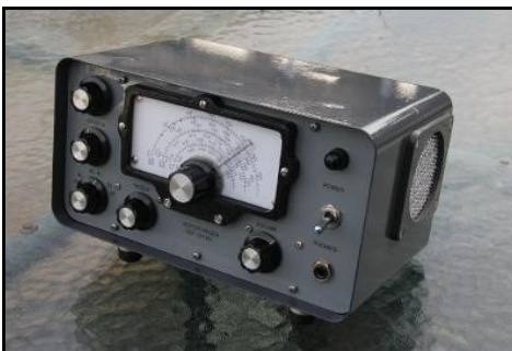
Nevell's "modern build" of the receiver section of the Hexter transceiver.
