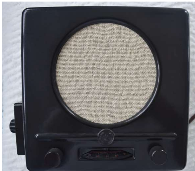
DKE: the last and cheapest radio made. 2 tubes, regen.
