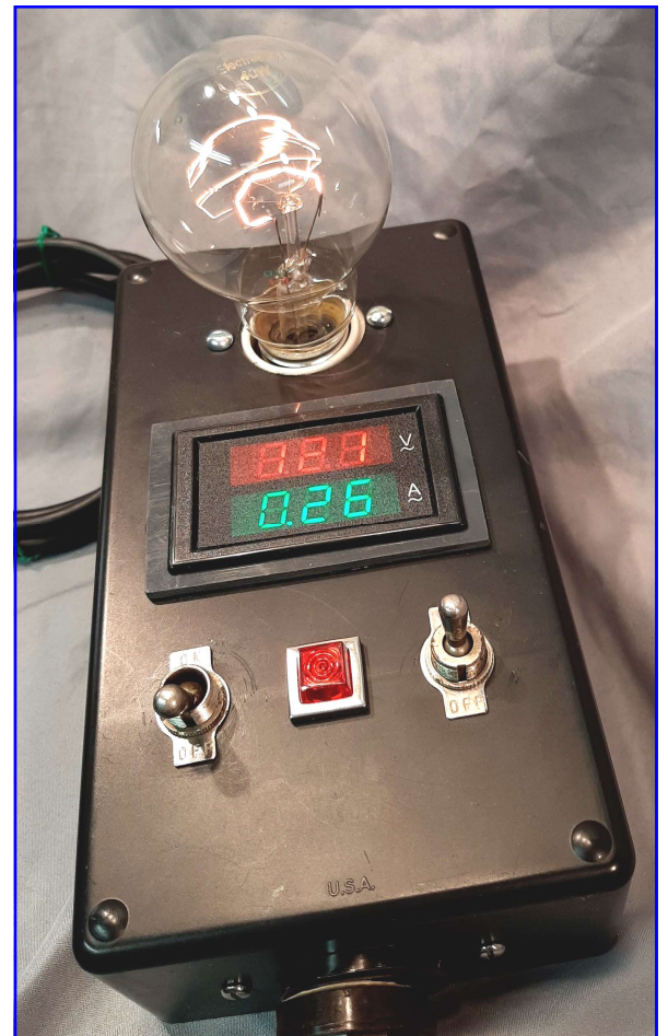
G.E model 422 6-tube series string radio is under test on startup. 121 VAC x 0.26 amperes = 31.46 watts lighting the 40 watt clear bulb briefly, then out as filaments come to operating temperature, proving there were no initial shorts in the radio.
