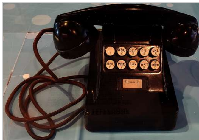
Prototype touch-tone phone. Notice the lack of # and *
