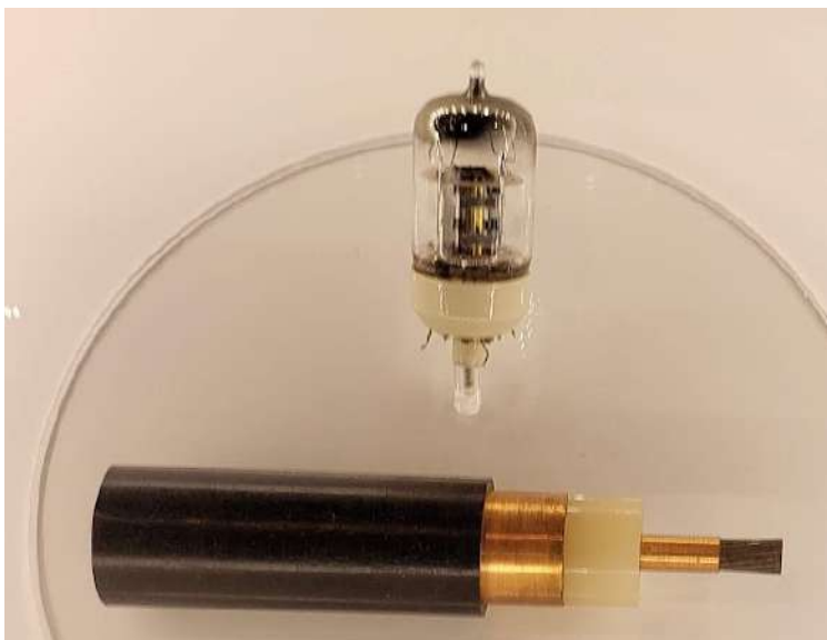
A piece of the 1956 Transatlantic cable with in-cable repeater tube
