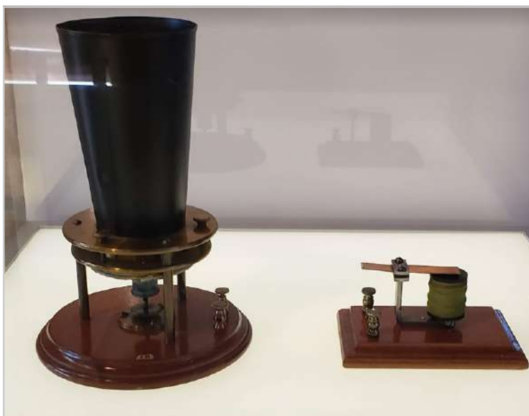
A replica of Alexander Graham Bell's 1876 prototype phone
