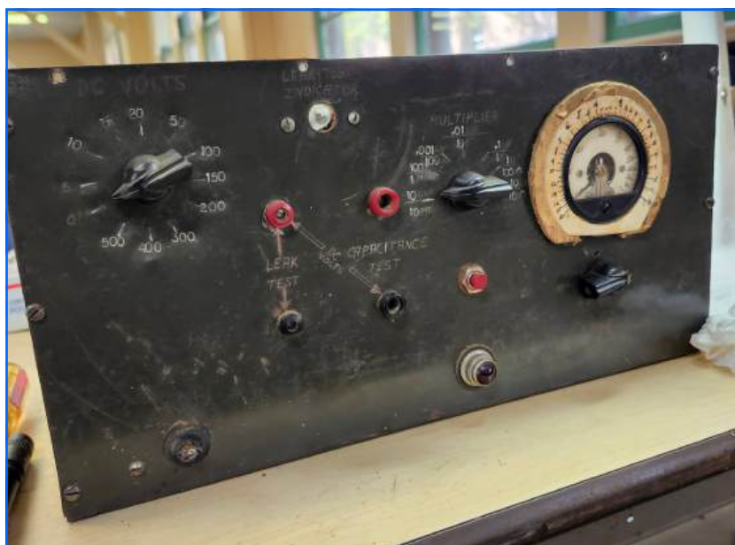
The Homebrewed Capacitor Checker
