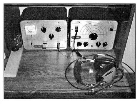
affair using the (then) popular 6DQ6B TV sweep tube. (For more than 10 years the transmitter in the ARRL's How to Become a Radio Amateur was based upon the same tube.) It is crystal controlled and has a power input of 25 W. The controls are very basic: ON/OFF, Band, Tune and Load. There is a crystal socket and a key jack on the front panel, an antenna jack on the back, and that's it.
