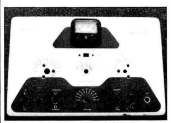
Figure A-A Heath DX-20 panel that required repair.
