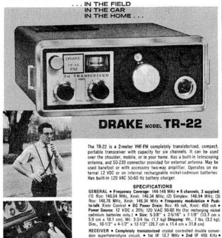
\*PRICE OF TR-22 INCLUDES: Dynamic Microphone, Over-the-Shoulder Carrying Case, 120 VAC and 12 VDC Power Cords, Speaker/Headphone Plug, and 10 Nickel-Cadmium Batteries. RECEIVER • Completely transistorized crystal controlled double conversion superheterodyne circuit. • 1st IF 19.7 MHz • 2nd IF 455 KHz • Antenna Input Impedance: 50 ohms • Sensitivity: .5 microvolt or less for 20 dB S+N/N ratio • Audio Output: 0.7 watt at 10% or less distortion • Built-in speaker.
