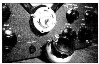
Detail of the homemade gear reduction assembly and hand-milled knob skirt for K's homebrew 75A-4.
