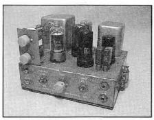
The Stancor ST-203-A with the cover removed
