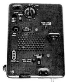
Figure 3—The RT-6 transmitted up to 10 W in two bands. The "A" model provided wideband capability.
