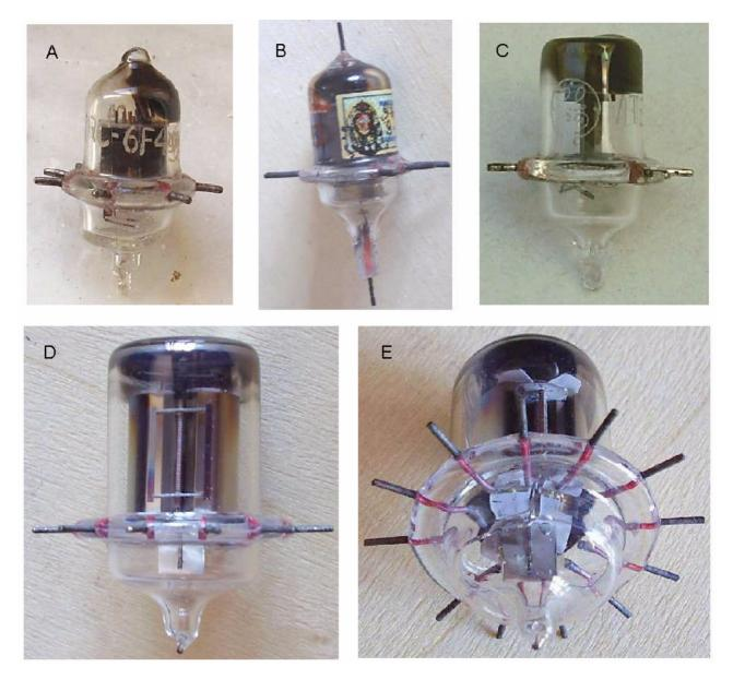
Acorn tubes were introduced around the mid 930s to reduce parasitic parameters, inductance and capacitance, of the connections. Pins went out radially from the glass press around the body and sometimes from the top and from the bottom. When the miniature 7 pin bulbs appeared, the small electrode structures of the acorn tubes were readily moved to the new envelope, without appreciable decrease in high frequency performances.
