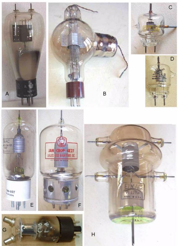
The VHF road in convection cooled transmitting tubes
