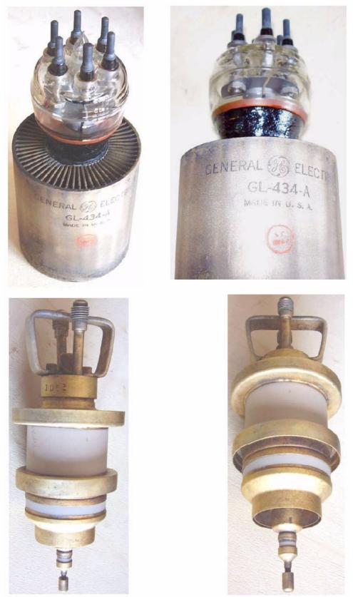
Two transmitting tubes from General Electric. GL-434-A was used in early radar applications. The coaxial tetrode GL-6019 delivers 1KW output at 900MHz. Water cooled, it was intended for UHF TV transmitters.
