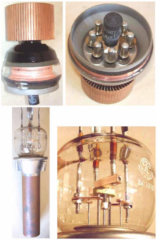
Here two British made power transmitting tubes. 4H-162E, on top, is rated for 500W anode dissipation with forced air cooling. CV28, bottom, requires external radiator. It is capable of 1.2KW anode power dissipation.
