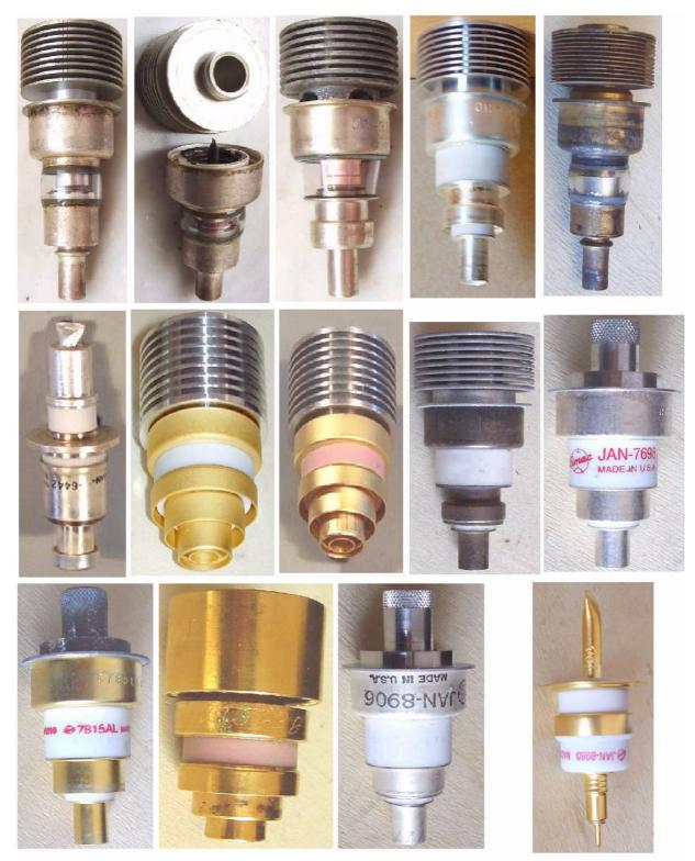
Oil-can tubes were introduced as a variant of planar tubes, to increase anode power dissipation. The anode is large and has either an integral radiator or a conductive surface to be mounted in some external cooler. Power dissipation in the order of 100W, with operating frequencies up to about 3GHz were available.
