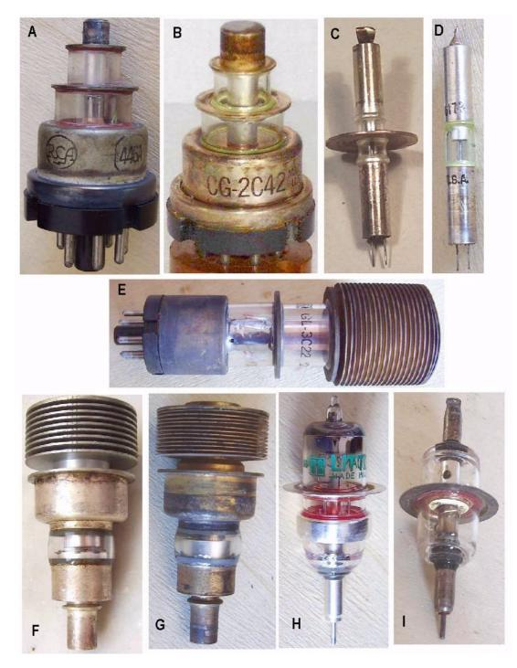
Operation in the UHF region around 1GHz and over required close spacing of electrodes: planar structures were simple enough to produce, once defined a reliable process of soldering the glass spacers, used in the early '940s, to electrode copper surfaces. Several shapes were designed depending upon the anode power dissipation and the mechanical interface to the external cavities. Useful frequency up to about 3GHz.
