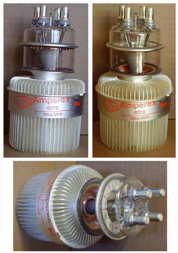
6076 is a forced air cooled transmitting tetrode. 3.5KW, 220MHz. Intended for FM-TV transmitters.
