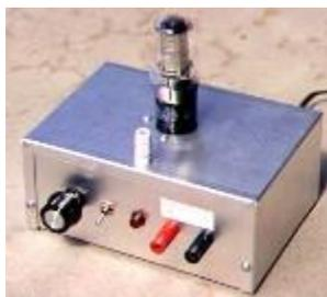
The voltage regulator requires a certain minimum current (about 5 mA) to function properly. If you are only drawing a few milliamperes from the supply, connect a 12k bleeder resistor across the output. Otherwise, the regulator will not adjust down to the lower voltages. Or, 220Ω and 10k fixed resistors, and a 15k pot, could be used at the voltage regulator, which would draw the necessary minimum current. The VR tube can be replaced by a high-voltage Zener diode.
