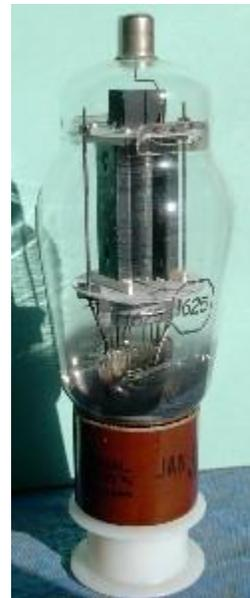
within its amateur (ICAS) or commercial (CCS) ratings. If a plate gets hotter than when it was outgassed at the evacuation of the tube, it may emit gases and ruin the tube.
