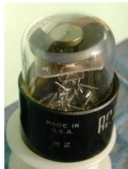
and octal base, in line with military standards, and this is the least expensive electron-ray tube at present, the others, where available, being more costly. The 6AF6/6AD6, a photograph of which is shown at the right, had two ray-control electrodes on opposite sides and no triode, while the 6AF7 had (it seems) twin sectors that moved concurrently. Finally, the 6AL7 had two rectangular displays that could be changed in size by control electrodes. These tubes are discussed below.
