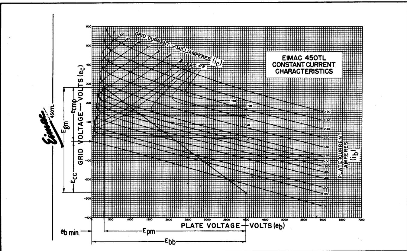
Figure 3. Method of determining  $e_{c \text{ mp}}$  and  $i_c$  on 450TL constant-current characteristics from values of  $e_{b \text{ min.}}$  and  $E_{pm}$  found in steps 6 and 7 and value of  $i_b$  found in step 10. The value of  $E_{cc}$  and  $E_{gm}$  from steps 13 and 14 and the operating line are also shown.
