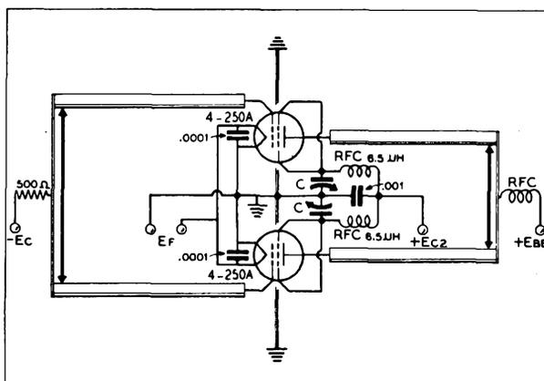
Screen-tuning neutralization circuit for use above 45 Mc.
