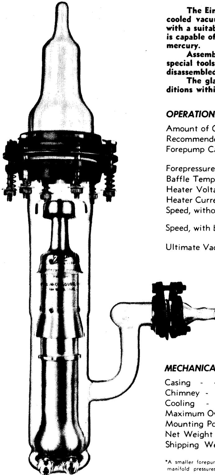
The Eimac HV-1 Diffusion Pump is a fast, triple-jet, air-cooled vacuum pump of the oil-diffusion type. When used with a suitable mechanical forepump and Eimac type A oil it is capable of reaching an ultimate vacuum of  $4 \times 10^{-7}$  mm of mercury.
