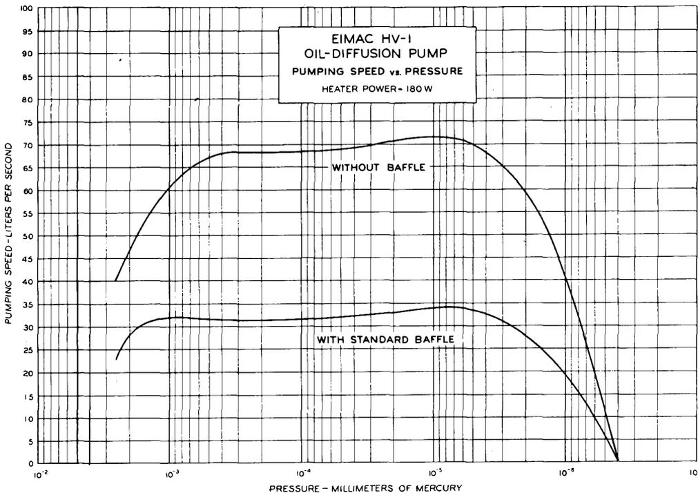
The curves at the left show the gas handling capabilities of the HV-1 over a range of pressures both with and without a baffle. These curves apply when a forepump with the required capacity is used. The rapid loss in pumping speed at the higher pressures is due to the inability of the forepump to handle the necessary volume of gas. With a larger forepump, the pumping speed would be maintained out to higher pressures.
