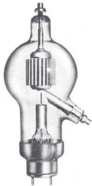
This 1500-watt medium- $\mu$  (24) triode is intended for use in general-purpose high-power applications at frequencies up to 40 megacycles. It is cooled by radiation and forced air.
