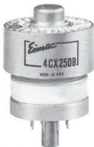
A 250-watt general-purpose external-anode tetrode featuring ceramic-metal construction. This compact power tube can be used at maximum ratings at frequencies up to 500 megacycles. It is recommended for use in equipments of new design.
