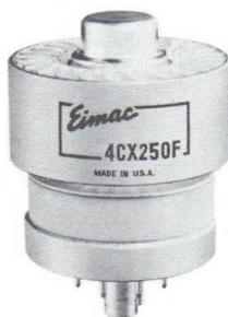
The 4CX250F is a ceramic and metal radial-beam tetrode with electrical characteristics similar to the 4CX250B but designed for use where a heater voltage of 26.5 volts is more desirable. Maximum ratings apply to 500 megacycles but the tube is also an excellent choice for other r-f or a-f applications. It is recommended for use in equipments of new design.
