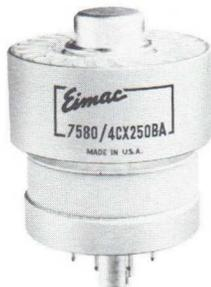
This new addition to the Eimac line of ceramic and metal tetrodes has high-gain characteristics which make it particularly suitable for class-AB<sub>1</sub> radio-frequency or audio-frequency service; of course, it is also an excellent power tetrode for class-C service. Maximum ratings apply at frequencies up to 500 megacycles.
