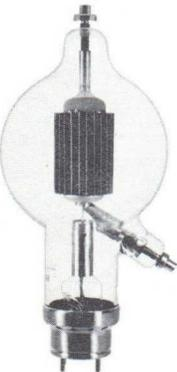
The largest internal-anode triode in the comprehensive Eimac line. The 2000T has a medium- $\mu$  (23) and is intended for high-power general-purpose service at frequencies through 40 megacycles. It is cooled by radiation and forced air.
