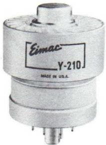
A special version of the ceramic and metal 4CX250B intended for use where small size and light weight are important. It may be cooled by liquid immersion or by the use of a suitable heat sink; maximum allowable plate dissipation is determined by the adequacy of the cooling supplied but in no case should it exceed 250 watts.
