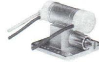
The Y-222 is a special version of the ruggedized, ceramic and metal 1K20-series reflex klystrons. This tube was designed primarily for use in mobile and fixed-station commercial carrier-system applications, and is capable of delivering a minimum output power of 70 milliwatts over the frequency range of 10.5-10.7 kilomegacycles.
