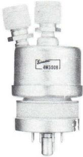
A general-purpose radial-beam tetrode with electrical characteristics similar to those of the Eimac 4X250B, this water-cooled version is intended for use where reserve anode dissipation is desired or where the use of water is a convenience. Maximum ratings apply to frequencies as high as 500 megacycles.
