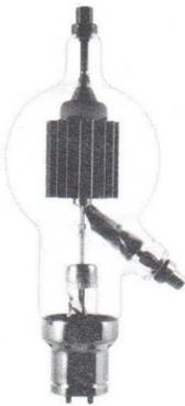
This high-power high- $\mu$  (35) triode enjoys a maximum plate-dissipation rating of 1000 watts; this and other maximum ratings apply through 50 megacycles. It is cooled by radiation and forced air.
