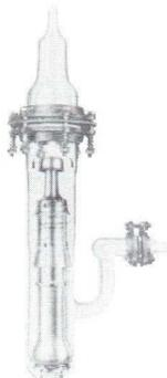
A fast, triple jet, air-cooled vacuum pump of the oil-diffusion type. When used with a suitable forepump and cold trap it is capable of reaching an ultimate vacuum better than  $10^{-7}$  mm of mercury.
