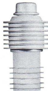
This tube type is a horizontally-finned version of the famous 4CX300A and is intended for use where transverse air cooling is desired. However, it is also useful in applications where anode power is dissipated by liquid immersion. Its electrical characteristics are identical to those of the 4CX300A with the exception of plate dissipation, which is established at 125 watts maximum when air cooling is employed. It is ideally suited for applications where shock and/or vibration are experienced.
