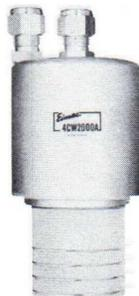
This recent addition to the Eimac line is electrically identical to the popular 4CX1000A except for its plate dissipation rating which is 2000 watts. It is intended for use where water cooling is preferred or where higher anode-dissipation capability is required.
