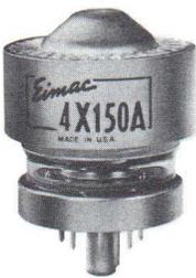
This veteran of external-anode tetrodes, and an Eimac original, continues to enjoy its deserved popularity. Recent tube improvements have made possible increases in maximum plate-voltage and plate-dissipation ratings. In class-AC or class-C service an input power of 500 watts is now allowed at frequencies up to 150 megacycles.
