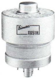
This version of the new 7580 ceramic and metal tetrode employs a 26.5-volt heater. Accordingly, it is especially recommended for applications where this supply voltage plus the high-gain characteristics of the 7580 are requisites.
