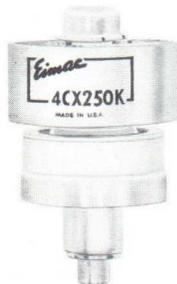
This coaxial-based tetrode is particularly useful as a CW r-f amplifier between 500 and 1200 megacycles; in pulse applications, its useful upper frequency is above 1500 megacycles. The 4CX250K requires a heater voltage of 6.0 volts; it is recommended for use in new equipment.
