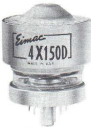
A 26.5-volt heater makes the 4X150D suitable for service in many applications where this somewhat unusual heater voltage is encountered. This tube type has recently been improved and it now carries new plate-voltage and plate-dissipation ratings; present ratings allow 500 watts input at frequencies up to 150 megacycles.
