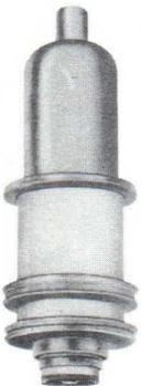
This very-high- $\mu$  triode, designed for use in klystron switch-tube applications, represents a new answer to the requirement for a high-voltage tube with moderate current-carrying capability. Its modulating anode, while requiring fairly high drive voltage, demands little in the way of drive power. It is usually cooled by immersion in oil or other suitable insulating liquid.
