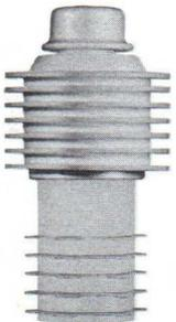
This special version of the horizontally-finned 4CX125C is nickel and rhodium plated to allow its immersion in liquids which are corrosive to silver. Of course, it may be used with forced-air cooling, in which case its plate dissipation rating is 125 watts. Its internal construction makes it a good choice for applications where shock and/or vibration are encountered.
