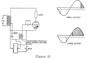
The small capacitor in the grid lead acts to generate a fixed d-c. bias by grid rectification. The functioning of the saturating transformer (a transformer fed from a voltage source higher than its normal voltage rating) through a series reactance (or resistance) is best understood by considering the primary current and flux shown in Fig. 32.
