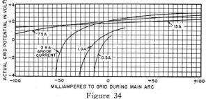
If any capacitances or inductances receive stored energy by reason of the grid current flow during this period, which is not dissipated before the next cycle, there is a carryover effect which appears to change the firing on the next cycle due to current flow on preceding cycles.
