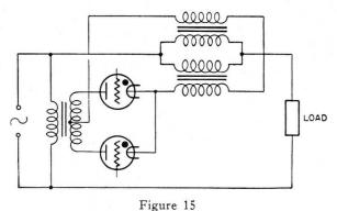
Figure 15 takes advantage of magnetic amplification to increase the KVA controlled with given tubes at the expense of speed of response. Amplification of the controllable power output of the tubes may be obtained, the amount depending largely on the allowable current when both tubes are shut off, and on the acceptable physical size of the reactor. Speed of response of the particular saturating reactor sets the d-c. supply requirements of the controlled rectifier.
