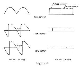
In the ideal case the d-c. meter value of the output voltage neglecting the small effect of overlap is:
