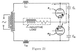
In this circuit the load inductance forces current to flow through the conducting tube (assumed #1 above) beyond the end of each positive half cycle by generating a voltage to more than oppose the voltage of the transformer secondary as it goes negative. This conduction continues until the grid circuit allows the next or "entering tube" (#2 above) to fire.
