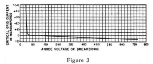
The critical grid current is a function of deionizing conditions as will be apparent from the consideration of deionization time. Therefore, the critical grid current immediately after each conduction cycle is greater than the grid current before the first cycle of conduction.
