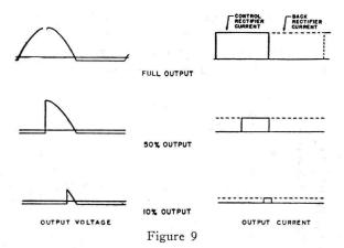
Peak forward voltage applied to the grid control tube and peak inverse voltage applied to the rectifier is 1.41 a-c. line voltage. Maximum output voltage is a-c. line voltage divided by 2.2 less tube drop. The d-c. meter value of current through the control tube and also that through the rectifier at full output is  $\frac{1}{2}$  the d-c. load current. See Fig. 9.
