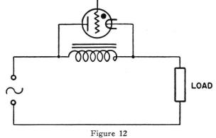
The circuit of Figure 12 utilizes the saturating effect of the d-c. component of current
