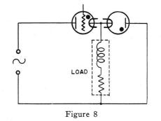
The above figure shows an additional circuit often used when the load is so highly inductive that current is always continuous. The load voltage is under control of the single grid.
