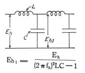
The voltage appearing across the capacitor of one section, is the input to the next section, which reduces this remainder by the same ratio, and so on through the filter. Supply frequency in the rectifier output due to trans-
