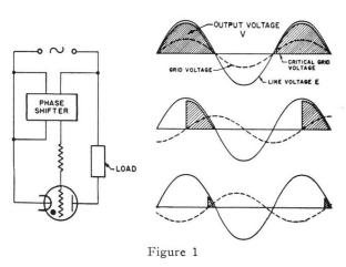
anode. The voltage between these electrodes is greater than the peak forward voltage by the amount of negative grid voltage. For this reason a maximum negative grid voltage rating is specified. Within limits a greater negative grid voltage may be applied if the peak forward voltage is correspondingly reduced.
