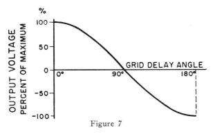
The negative output voltage range in Figure 7 occurs with grid retard greater than 90°, since the negative area under the output voltage curve exceeds the positive. Such operation requires a source of d-c. voltage to force current flow and constitutes the region where the unit operates as an inverter, supplying power to the a-c. lines.
