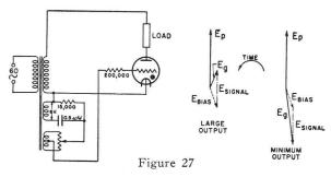
(b) Adding a variable polarity and magnitude d-c. grid voltage to a fixed a-c. bias voltage ("rider") which lags the anode voltage approximately 90° (Fig. 28). Normally voltages of less than 5 volts for the a-c. bias should be avoided.
