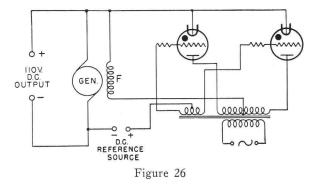
It might be noted that the effect on the tube firing is the same if a number of grid voltages are added in series and the sum applied through a current limiting resistance to one grid, or if a number of grids are placed in sequence across the discharge path in the tube and each voltage applied to a grid.
