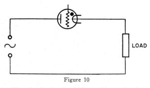
The simple circuit of Figure 10 may be shut off completely or turned on to give a pulsating d-c. output with an rms voltage of 71% of the a-c. supply less tube drop allowance. Due to the a-c. form factor the tube can pass an rms. current of 157% of its d-c. rating without overload. Peak forward voltage is 1.41 times a-c. line voltage plus allowances. If a transformer is used the magnetic circuit usually requires an air gap to prevent saturation by the d-c. component of primary current.
