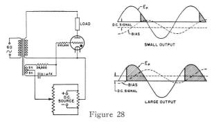
It is of interest to note that for the special case of a single phase full wave rectifier supplying inductive load, an in-phase rider rather than a 90° lagging rider is permissible since nearly the full range of control is obtained between  $0^{\circ}$  and  $90^{\circ}$  of grid retard.
