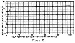
Above approximately 10V an arc is established to the grid. A steady arc drop appears between grid and cathode, and any remaining voltage is absorbed in other parts of the grid circuit.
