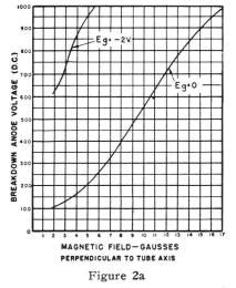
slightly from the above since some filament voltage is effectively in the grid circuit. The critical grid voltage is affected to some extent by magnetic fields in the cathode anode region of the tube. To indicate the order of magnitude the curves in Fig. 2a & 2b give the test results on a representative EL C6J tube.
