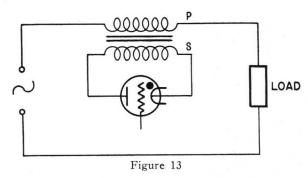
Figure 13 allows the use of the most efficient voltage for the tube regardless of line voltage. For this circuit tube voltage factors for Figure 12 should be divided by N (the ratio of primary to secondary turns). The tube current is in the order of 0.9N. or less, times the a-c. line current when the tube is fired full on.
