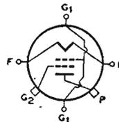
May be operated in vertical position only with grid-No.1 and filament terminals up. OUTLINE 93, Outlines Section.
