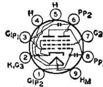
equipment operating at frequencies up to 500 Mc. Tube is internally neutralized for push-pull amplifier service. At 500 Mc, tube delivers useful power output of 5 watts in CCS or 6 watts in ICAS.
