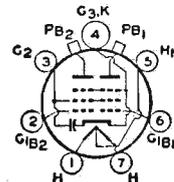
Heater-cathode type containing two high-perveance units used as rectangular-wave pulse modulator. Modulator Service maximum CCS plate dissipation (per tube), 15 watts. Requires Septar seven-contact socket and may be operated in vertical position with base up or down, or in horizontal position with pins 2 and 6 in horizontal plane. OUTLINE 22, *Outlines* Section. Plates show no color when the tube is operated at maximum CCS ratings.
