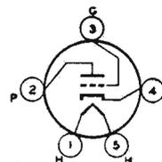
Heater-cathode type used as rf power amplifier and oscillator. May be used with full input up to 6 Mc and with reduced input up to 30 Mc. Requires Small five-contact socket and may be operated in any position. OUTLINE 32, *Outlines* Section. Heater volts (ac/dc), 2.5; amperes, 2.5. Direct interelectrode capacitances: grid to plate, 3.9  $\mu\text{f}$ ; grid to cathode and heater, 4  $\mu\text{f}$ ; plate to cathode and heater,
