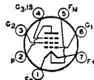
Seven-pin miniature type having quick-heating, mid-tapped, coated filament used as af power amplifier and modulator, rf power amplifier and oscillator, and frequency multiplier in
