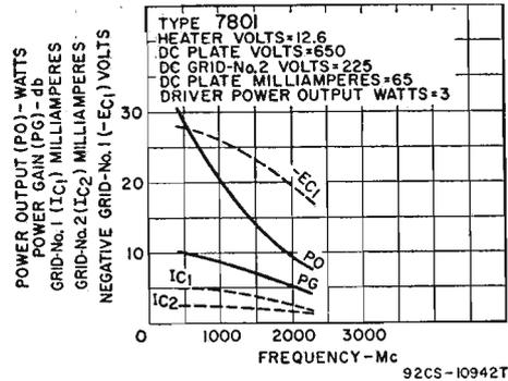
PLATE-MODULATED RF POWER AMPLIFIER—Class C Telephony
