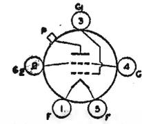
Forced-air-cooled, thoriated-tungsten-filament type used as af power amplifier and modulator and as rf power amplifier and oscillator. May be used with full input up to 30 Mc
