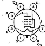
at 120 Mc, plate voltage and plate input should be reduced to 75 per cent of maximum ratings. Class C Telegraphy maximum plate dissipation, CCS 21 watts, ICAS 25 watts. Requires Octal socket and may be operated in any position. OUTLINE 21, *Outlines* Section.
