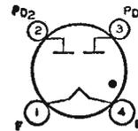
Coated-filament, glass type used to supply dc power of uniform voltage to receivers in which the rectified current requirements are subject to considerable variation. Tube requires four-contact socket and should be operated in vertical position with base down. OUTLINE 32, Outlines Section. Maximum peak inverse plate volts, 1550; maximum peak plate amperes (per plate), 1.
