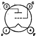
Thoriated-tungsten-filament type used as af power amplifier and modulator. Requires Small four-contact socket and may be operated in vertical position with base down, or in horizontal position with pins 1 and 4 in vertical plane. OUTLINE 32, *Outlines* Section. Filament volts (ac/dc), 7.5; amperes, 1.25. Direct interelectrode capacitances: grid to plate, 6.4  $\mu\text{f}$ ; grid to filament, 3.2  $\mu\text{f}$ ; plate to filament, 2.6
