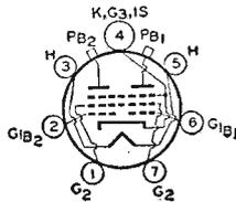
to 100 Mc and with reduced input up to 470 Mc. Class C Telegraphy maximum plate dissipation (per tube), CCS 20 watts, ICAS 25 watts. Requires Septar seven-contact socket and may be operated in any position. OUTLINE 14, *Outlines* Section. Heater volts (ac/dc), 12.6; amperes, 0.625. Except for heater rating, the 6850 is identical with type 6524.
