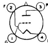
capacitances: grid to plate, 9.25  $\mu\text{f}$ ; grid to filament, 6  $\mu\text{f}$ ; plate to filament, 5  $\mu\text{f}$ . Plate shows a barely perceptible red color when tube is operated at maximum CCS ratings. Except for interelectrode capacitances, the 835 is identical with DISCONTINUED type 211. The 835 is a DISCONTINUED type listed for reference only.
