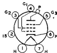
per cent of maximum ratings; at 60 Mc, to 62 per cent. Class C Telegraphy maximum CCS plate dissipation, 12 watts. Requires Medium seven-contact socket and may be operated in any position. OUTLINE 34, *Outlines* Section, except has no bayonet pin. Plate shows no color when tube is operated at maximum CCS ratings.
