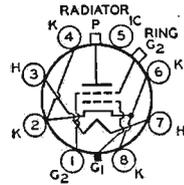
equipment. May be used with full input up to 500 Mc. Maximum plate dissipation for either service, CCS 250 watts.
