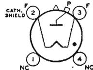
Super-Jumbo four-contact socket and may be operated in vertical position only, base down. OUTLINE 56, *Outlines* Section. Except for physical dimension and base, the 8008 is identical to type 872A.
