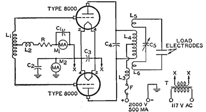
C<sub>1</sub> C<sub>2</sub> C<sub>3</sub> = 0.005 μf, mica, 600 v.
