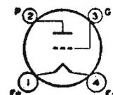
up to 120 Mc. Class C Telegraphy maximum plate dissipation, CCS 20 watts. Requires Small four-contact socket and may be operated in vertical position with base down, or in horizontal position with pins 1 and 4 in vertical plane. OUTLINE 32, *Outlines* Section. Plate shows no color at maximum CCS ratings.
