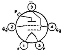
natural cooling, or 75 Mc with forced-air cooling and with reduced input up to 120 Mc. Class C Telegraphy maximum CCS plate dissipation, 250 watts. Requires Special Metal-Shell Giant five-contact socket and may be operated in vertical position only, base up or down. OUTLINE 40, *Outlines* Section. Plate shows an orange-red color when the tube is operated at maximum CCS ratings.
