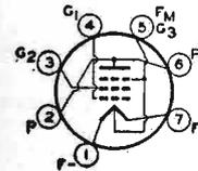
Seven-pin miniature type having coated filament used as rf power amplifier in light-weight, compact, portable, low-power, battery-operated equipment. May be used at full input up to 10 Mc. Class C maximum CCS plate dissipation, 2 watts.
