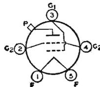
Telegraphy maximum CCS plate dissipation, 400 watts. Requires Special Metal-Shell Giant five-contact socket and may be operated in vertical position only, base up or down. OUTLINE 40, *Outlines* Section.
