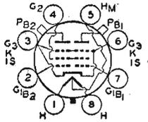
and plate input should be reduced to 80 per cent of maximum ratings; at 200 Mc, to 70 per cent. Class C Telegraphy maximum plate dissipation (per tube), CCS 20 watts, ICAS 25 watts. Requires Octal socket and may be operated in any position. OUTLINE 24, *Outlines* Section. Plates show no color when tube is operated at maximum CCS or ICAS ratings.
