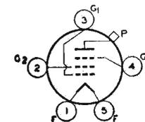
Thoriated-tungsten-filament type used as rf power amplifier and oscillator. May be used with full input up to 15 Mc and with reduced input up to 80 Mc. Class C Telegraphy maximum plate dissipation, CCS 40 watts, ICAS 50 watts. Requires Small five-contact socket and may be operated in vertical position with base down, or in horizontal position with pins 2 and 4 in vertical plane. OUTLINE 51, *Outlines* Section.
