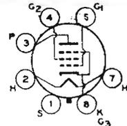
should be reduced to 90 per cent of maximum ratings; at 90 Mc, to 85 per cent. Class C Telegraphy maximum CCS plate dissipation, 10 watts. Requires Octal socket and may be operated in any position. OUTLINE 11, *Outlines* Section.
