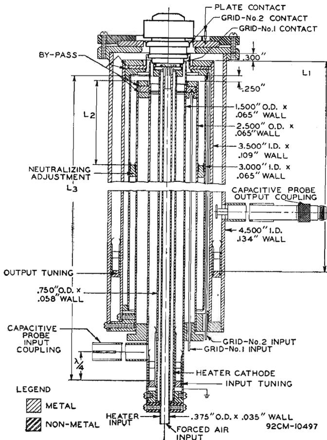
$L_1$  = Length of Grid-No.2-Plate Cavity, 1 to 20 inches, approx., depending on frequency and mode
