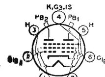
Small, sturdy, heater-cathode type used as af power amplifier and modulator, as push-pull rf power amplifier and oscillator, and as frequency tripler. May be used with full input up to 100
