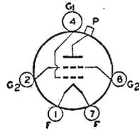
maximum CCS plate dissipation, 65 watts. Requires Septar seven-contact socket and may be operated in vertical position only, base up or down. OUTLINE 23, Outlines Section. Plate shows an orange-red color when the tube is operated at maximum CCS ratings.
