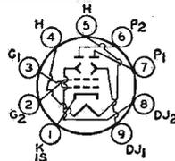
Used for modulator, demodulator, and frequency-converter applications in single- and double-sideband, suppressed-carrier communications equipment operating at frequencies up to 100 Mc; used with single-ended or push-pull input to provide push-pull balanced output; used in low-cost balanced-modulator, balanced-mixer, and product-detector service.
