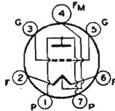
to filament, 1.1 μf. Maximum CCS ratings as RF POWER AMPLIFIER AND OSCILLATOR, Class C Telegraphy with forced-air cooling: dc plate volts, 1000 max; dc grid volts, -600 max; dc plate milliamperes, 125 max; dc grid milliamperes, 40 max; plate input, 125 max watts; plate dissipation, 60 max watts. Plate shows an orange-red color when tube is operated at maximum CCS ratings. The 826 is a DISCONTINUED type listed for reference only.
