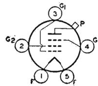
duced to 80 per cent; at 75 Mc, to 64 per cent. Class C Telegraphy maximum plate dissipation, CCS 50 watts, ICAS 65 watts. Requires Small five-contact socket and may be operated in vertical position with base down, or in horizontal position with pins 2 and 4 in vertical plane. OUTLINE 51, *Outlines* Section. Plate shows no color when tube is operated at maximum CCS ratings, and shows a barely perceptible red color at maximum ICAS ratings.
