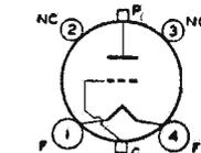
be reduced to 80 per cent of maximum ratings; at 350 Mc, to 53 per cent. Class C Telephony maximum CCS plate dissipation, 50 watts. Requires Small four-contact socket and may be operated in vertical position only, base up or down. OUTLINE 47, *Outlines* Section. Plate shows an orange-red color when tube is operated at maximum CCS ratings.
