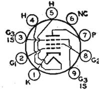
quency-multiplier service at frequencies up to 40 Mc; also used in modulator and af power-amplifier applications. Requires Miniature nine-contact socket and may be operated in any position. OUTLINE 6, *Outlines* Section. During manufacture, this tube is subjected to special controls and tests for heater-cycling, heater-cathode leakage, interelectrode leakage, low-frequency-vibration performance, 500-hour intermittent life performance, and intermittent shorts.
