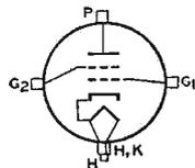
shock and vibration is essential. May be used with full input up to 1215 Mc, and with reduced efficiency at higher frequencies. Plate-and-Screen Pulsed RF Amplifier maximum average plate dissipation, CCS 600 watts; maximum pulse duration, 10 microseconds in any 1000-microsecond interval. Tube has matrix-type cathode.
