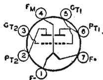
full input up to 40 Mc. Class C Telegraphy maximum CCS plate dissipation (each unit), 1 watt. Requires miniature seven-contact socket and may be operated in any position. OUTLINE 5, *Outlines* Section. For filament considerations, refer to type 3A4, noting that for type 3A5 pin 4 is the filament mid-tap. Plates of the 3A5 show no color when the tube is operated at CCS ratings.
