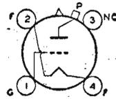
operation at 45 Mc, plate voltage and plate input should be reduced to 82 per cent of maximum ratings; at 80 Mc, to 55 per cent. Class C Telegraphy maximum CCS plate dissipation, 125 watts. Requires Jumbo four-contact socket and may be operated in vertical position with base down, or in horizontal position with pins 1 and 3 in vertical plane. OUTLINE 53, Outlines Section. Plate shows no color when tube is operated at maximum CCS ratings.
