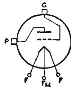
ment, 3.2  $\mu f$ . Maximum CCS ratings as RF POWER AMPLIFIER AND OSCILLATOR: dc plate volts, 3000 max; dc grid volts, -500 max; dc plate milliamperes, 500 max; dc grid milliamperes, 150 max; plate input, 1500 max watts; plate dissipation 600 max watts. The 6C24 is a DISCONTINUED type listed for reference only. As a replacement, the 5786 is a similar type although not directly interchangeable.
