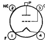
Thoriated-tungsten-filament type used as rf power amplifier and oscillator. May be used with full input up to 60 Mc and with reduced input up to 120 Mc. Class C Telegraphy maximum
