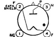
Coated-filament type used in power supply of transmitting and industrial equipment. Maximum peak inverse anode volts, 15000; maximum average anode amperes, 1.5. Requires
