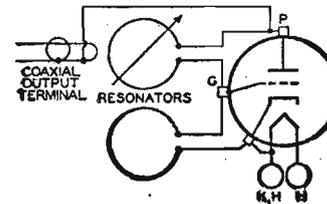
temperatures ranging from -55 to +75°C. UHF Oscillator maximum plate dissipation, 3.6 watts.
