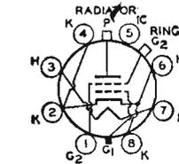
legraphy maximum CCS plate dissipation, 250 watts. Full ratings to 150 Mc; reduced ratings to 500 Mc. May be operated in any position. OUTLINE 82, *Outlines* Section. Air flow must be adequate to limit the plate and seal temperatures to their specified maximum values. A minimum air flow of 5.3 cfm must pass through the radiator. Less air flow is required when an air-system socket is used to direct the flow of air through the radiator.
