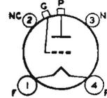
Thoriated-tungsten-filament type used as rf power amplifier and oscillator. May be used with full input up to 30 Mc and with reduced input up to 130 Mc. Requires Small four-contact socket and may be operated in vertical position only, base down. Maximum over-all length, 6-1/16 inches; maximum diameter, 2-3/16 inches. Filament volts (ac/dc), 7.5; amperes, 4. Direct interelectrode capacitances:
