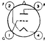
operated in vertical position with base down, or in horizontal position with pins 1 and 3 in vertical plane. OUTLINE 52, *Outlines* Section. Plate shows no color when tube is operated at maximum CCS ratings.
