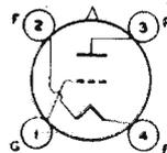
Thoriated-tungsten-filament type used as af power amplifier and modulator and as rf power amplifier and oscillator. May be used with full input up to 30 Mc and with reduced input up to 120 Mc. Requires Jumbo four-contact socket and may be operated in vertical position with base down, or in horizontal position with pins 1 and 3 in vertical plane. OUTLINE 52, *Outlines* Section. Plate shows no color when tube is operated at maximum CCS ratings. The 838 is used principally for renewal purposes.
