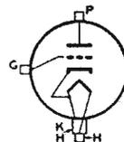
Forced-air-cooled heater-cathode type having integral radiator used in cathode-drive circuits as rf power amplifier and oscillator. May be used with full input up to 1200 Mc and at reduced ratings up to 2000 Mc. Type 5588 may be operated in vertical position only, radiator up or down. OUTLINE 89, *Outlines* Section. A minimum air flow of 10 cubic feet per minute should be directed through the radiator toward
