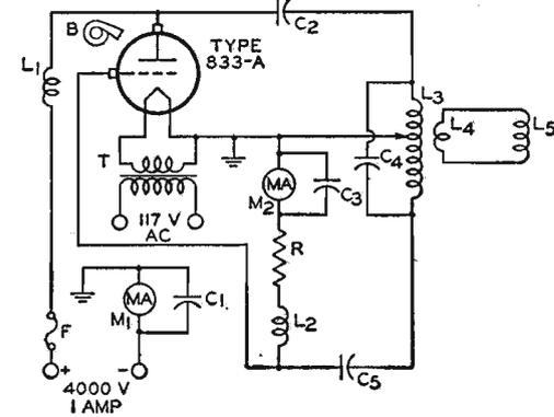
C<sub>1</sub> C<sub>3</sub> = 0.01 μf, mica, 600 v.
