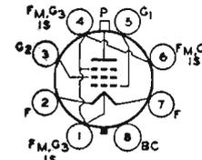
equipment. May be used with full input up to 125 Mc and with reduced input up to 175 Mc. Class C Telegraphy maximum plate dissipation, CCS 10 watts, ICAS 13.5 watts.
