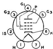
Mc, plate voltage and plate input should be reduced to 77 per cent of maximum ratings; at 100 Mc, to 55 per cent. Class C Telegraphy maximum plate dissipation, CCS 10 watts, ICAS 13 watts. Requires Medium seven-contact socket and may be operated in any position. OUTLINE 34, *Outlines* Section. Plate shows no color when the tube is operated at maximum CCS or ICAS ratings.
