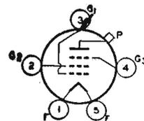
Thoriated-tungsten-filament type used as rf power amplifier and oscillator. May be used with full input up to 20 Mc and with reduced input up to 60 Mc. Class C Telegraphy maximum plate dissipation, CCS 125 watts. Requires Giant five-contact socket and may be operated in vertical position with base up or down, or in horizontal position with pins 2 and 5 in horizontal plane. OUTLINE 59, *Outlines* Section. Plate
