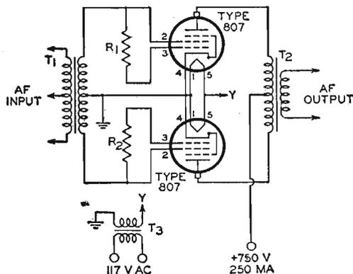
R<sub>1</sub> R<sub>2</sub>=20000 ohms, 1 watt, carbon
