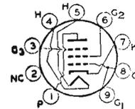
Nine-pin miniature heater-cathode type used as rf power amplifier and oscillator and as frequency multiplier. May be used with full input up to 50 Mc. Class C Telegraphy maximum plate dissipation, CCS 12 watts, ICAS 13.5 watts. Requires Noval nine-contact socket and may be operated in any position. OUTLINE 9, *Outlines* Section.
