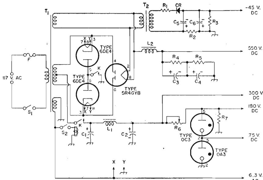
C<sub>1</sub> C<sub>2</sub> C<sub>3</sub> C<sub>4</sub> = 40 μf, electrolytic, 450 v.
