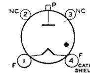
Coated-filament type used in power supply of transmitting and industrial equipment. Maximum peak inverse anode volts, 7500; maximum average anode milliamperes, 125. Re-
