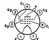
imum CCS plate dissipation, 125 watts. Requires Giant seven-contact socket and may be operated in vertical position only, base up or down. OUTLINE 38, Outlines Section. Plate shows a cherry-red color when the tube is operated at maximum CCS ratings.
