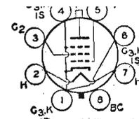
Small, sturdy, heater-cathode type used as af power amplifier and modulator and as rf power amplifier and oscillator. May be used with full input up to 60 Mc and with reduced input up to 175 Mc. Class C Telegraphy maximum plate dissipation, CCS 20 watts, ICAS 25 watts. Requires Octal socket and may be operated in any position. OUTLINE 18, *Outlines* Section. Heater volts (ac/dc), 12.6; amperes, 0.625. Except for heater rating and base, the 6883 is identical with type 6146.
