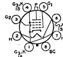
Small, sturdy, heater-cathode type used as rf power amplifier and modulator and as rf power amplifier and oscillator. May be used with full input up to 125 Mc and with reduced input up to 175 Mc. Class C Telegraphy maximum plate dissipation, CCS 10 watts, ICAS 13.5 watts. Requires Octal socket and may be operated in any position. OUTLINE 15, *Outlines* Section. Heater volts (ac/dc), 12.6; amperes, 0.4. Except for heater rating, the 6893 is identical to the 2E26.
