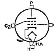
Small, sturdy, uhf, forced-air cooled, heater-cathode, cermolox type used as af power amplifier and modulator, and rf power amplifier and oscillator in compact and mobile and fixed equipment. Useful at frequencies up to 2000 Mc and beyond. Class C Telegraphy maximum plate dissipation, CCS 115 watts. May be operated in any position. OUTLINE 78, *Outlines* Section. Heater volts (ac/dc), 26.5; amperes, 0.52. Except for heater rating, the 6884 is identical with type 6816.
