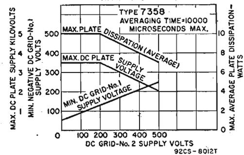
† Duty factor for the 7358 is defined as the ON time in microseconds divided by 10,000 microseconds. ON time is defined as the sum of the durations of all the individual pulses which occur during any 10,000-microsecond interval.
