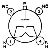
amperes, 0.25. Requires Small four-contact socket and may be operated in any position. OUTLINE 44, *Outlines* Section. The 836 has two separate cathodes, each of which is connected to its respective heater terminal. Plate-circuit return should be made to the mid-tap of the heater transformer.
