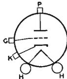
60,000 feet without pressurized chambers and under severe vibration conditions. May be used with full input up to 500 Mc and with reduced input up to 1700 Mc. Class C Telegraphy maximum plate dissipation, CCS 8 watts, ICAS 13 watts. The 6264A may be operated in any position. OUTLINE 72, *Outlines* Section. For other considerations refer to types 6263 and 6263A. The 6264 is a DISCONTINUED type listed for reference only. As a replacement, the 6264A is directly interchangeable.
