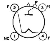
Thoriated-tungsten-filament type used in power supply of transmitting and industrial equipment. Requires Jumbo four-contact socket and may be mounted in vertical position, base down, or in horizontal position with pins 1 and 3 in vertical plane. OUTLINE 53, Outlines Section. Filament volts (ac), 10; amperes, 3.25.
