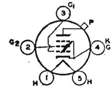
80 Mc, plate voltage and plate input should be reduced to 80 per cent of maximum ratings; at 125 Mc, to 55 per cent. Class C Telegraphy maximum plate dissipation, CCS 25 watts, ICAS 30 watts. Requires Small five-contact socket and may be operated in any position. OUTLINE 34, Outlines Section, except has no bayonet pin. Plate shows no color when tube is operated at maximum CCS or ICAS ratings.
