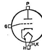
Forced-air-cooled type used as rf power amplifier and oscillator. May be used at full input up to 2500 Mc in cathode-drive circuits of the coaxial-cylinder type. Class C Telegraphy maximum CCS plate dissipation, 100 watts. May be operated in any position. OUTLINE 86, *Outlines* Section. Adequate air must be provided to prevent the temperature of the seals and the radiator from exceeding 250°C.
