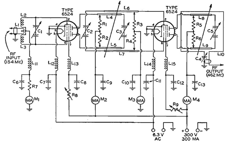
$C_1$   $C_2$  = 2.2-8.0  $\mu$ f per section, variable, butterfly, air gap 0.017 inch, Johnson 9MB11 or equivalent
