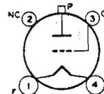
6.8; amperes, 2.5. Direct interelectrode capacitances: grid to plate, 6.7 µµf; grid to filament, 5.2 µµf; plate to filament, 0.9 µµf. Maximum CCS ratings as RF POWER AMPLIFIER AND OSCILLATOR: dc plate volts, 750 max; dc grid volts, -200 max; dc plate ma., 100 max; dc grid ma., 25 max; plate input, 75 max watts; plate dissipation, 25 max watts. Plate does not show color when tube is operated at maximum CCS ratings. Type 1623 is a DISCONTINUED type listed for reference only.
