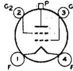
OSCILLATOR: dc plate volts, 750  $\text{max}$ ; dc grid-No.2 volts, 175  $\text{max}$ ; dc grid-No.1 volts, -200  $\text{max}$ ; dc plate ma., 60  $\text{max}$ ; dc grid-No.1 ma., 15  $\text{max}$ ; plate input, 45  $\text{max}$  watts; grid-No.2 input, 3  $\text{max}$  watts; plate dissipation, 15  $\text{max}$  watts. The 865 is a DISCONTINUED type listed for reference only.
