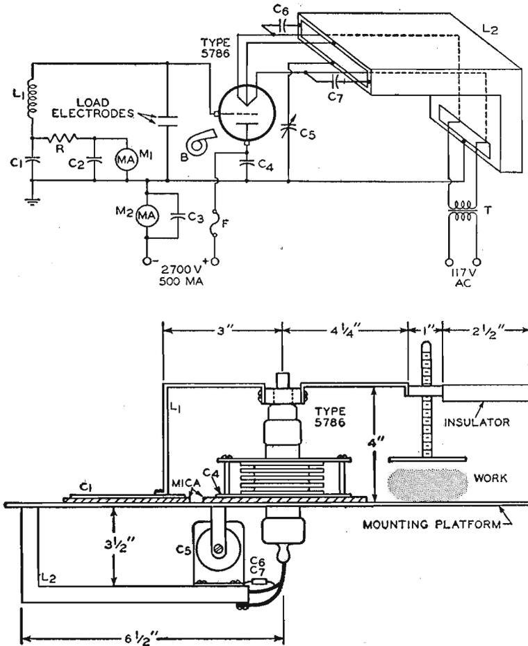
C<sub>1</sub>=250  $\mu$ f, mica 0.005 inch thick, 3 inches x 3 3/4 inches copper plate, held to mounting platform by insulated pressure clamps
