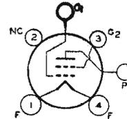
Thoriated-tungsten-filament type used as rf power amplifier and oscillator. May be used with full input up to 30 Mc. For operation at 60 Mc, plate voltage and plate input should be reduced to 75 per cent of maximum ratings; at 120 Mc, to 50 per cent. Requires Small four-contact socket and may be operated in vertical position only, base down. OUTLINE 57, *Outlines* Section. Plate shows no color when tube is operated at maximum CCS ratings. The 860 is used principally for renewal purposes.
