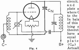
circuit. Figures 5 and 6 illustrate plate neutralization, where CN is returned to the plate circuit. In balanced circuits of this type, neutralizing condenser CN theoretically should have a capacitance equal to the gridplate capacitance ( $C_{\rm TP}$ ) of the tube. Actually, however, the correct value for
