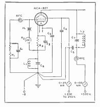
C<sub>1</sub>=0.001  $\mu$ f, mica C<sub>2</sub> C<sub>3</sub> C<sub>4</sub> C<sub>5</sub>=0.01  $\mu$ f, mica C<sub>6</sub>=100  $\mu\mu$ f midget C<sub>7</sub>=1.0  $\mu\mu$ f /meter R<sub>1</sub>=75000 ohms, 1 watt R<sub>2</sub>=2.0-Volt, 60-ma. pilot lamp R<sub>3</sub>=400 Ohms, 5 watts XL=Crystal of frequency "f" L<sub>4</sub>=See Note\* L<sub>2</sub>=Tune for f, 2f, or 4f
