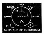
Tube Mounting Position VERTICAL-Base down. HORIZONTAL-Plane of electrodes vertical.
