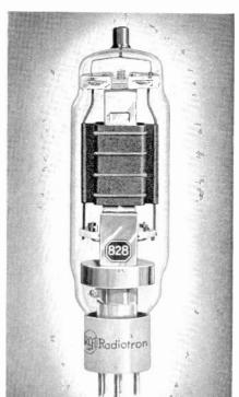
RCA-828 is also well suited for use as a class AB1 modulator and a-f power amplifier. Two tubes in class AB1, CCS, are capable of delivering 300 watts of audio power with only 1% distortion!
