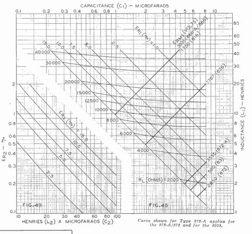
ing two type 866-A/866's, design a double-section filter which will limit the output ripple voltage to 0.5% at a load current equal to the combined maximum d-c load-current rating of the tubes (500 ma.) and still prevent the peak plate current of either tube from rising higher than its maximum peak plate-current rating. The input choke is to be of the swinging type and the voltage regulation is to be good from no-load to full load.
