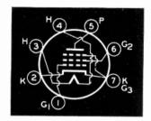
Bottom View of 9001 and 9003 Socket Connections
