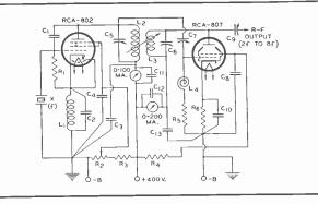
NOTE: Adjust coupling of L2 and L3 for maximum harmonic output. Correct polarization of L2 and L3 is essential.
