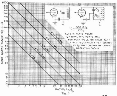
employed for the plate, or output, circuit of vacuum-tube r-f amplifiers, except at ultra-high radio frequencies, considerations involving inductance (L) and capacitance (C) are very important in transmitter design.
