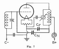
equal to that of the grid-plate neutralizing condenser.
