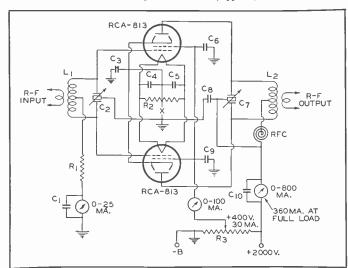
$C_1 C_8 C_4 C_6 C_{10} = 0.002 \ \mu f mica$  $C_2 = 2 \ \mu \mu f/meter/section$ Ce Co=0.05 µf mica, 1000 volts C7=1.5 µµf/meter/section C==0.005 µf mica, 2500 volts L1 L2=Tune to operating frequency or other means.
