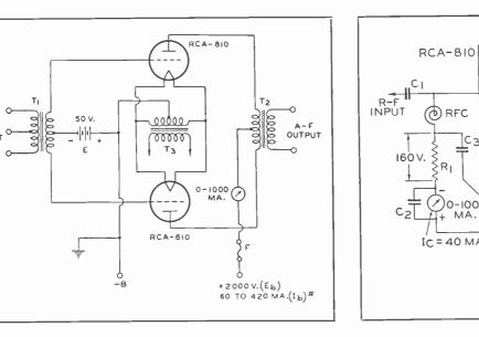
T1=Input transformer; plate-to-plate impedance, 1500 ohms (Note 2)
