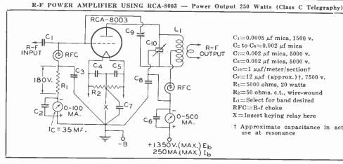
C1=0.0005 µf mica, 1500 v.  $C_2$  to  $C_6 = 0.002 \ \mu f$  mica C7=0.002 µf mica, 5000 v.  $C_8 = 0.002 \ \mu f mica, 5000 \ v.$ C10=1 µµf/meter/section† Co=12 µµf (approx.) +, 7500 v. R<sub>1</sub>=5000 ohms, 20 watts R2=50 ohms, c.t., wire-wound L1=Select for band desired RFC=R-f choke X=Insert keying relay here † Approximate capacitance in actual
