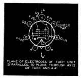
Tube Mounting Position VERTICAL—Plate terminals up or down. HORIZONTAL—Plane of each plate vertical (on edge). PIN 1=Heater PIN 2=Grid No. 1 of Unit No. 2 PIN 3=Screen PIN 4=Cathode PIN 5=Heater center tap PIN 5=Heater center tap PIN 6=Grid No. 1 of Unit No. 1 PIN 7 - Heater PunAnD Pug=Plate terminals of Units ULTRA-HIGH-FREQUENCY PLATE-MODULATED PUSH-PULL R-F POWER AMPLIFIER
