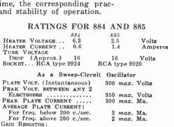
Should be not less than 1000 ohms per max, instantaneous volt applied to the grid. Values in excess of 0.5 megohm may cause circuit instability.
