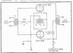
$T_1$ =Input transformer  $T_2$ =Output transformer; primary impedance 11600
