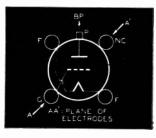
**Tube Mounting Position** VERTICAL-Base down. HORIZONTAL—Plane of electrodes vertical (on edge).
