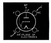
**Tube Mounting Position** VERTICAL—Base down only. HORIZONTAL—Plane of electrodes vertical.
