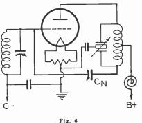
The neutralizing circuits shown in Figs. 5 and 6 are the ones most commonly used in amateur transmitters employing single-tube amplifier stages. They are entirely satisfactory for most transmitting triodes operating at frequencies up to 15 or 20 Mc. These circuits may cause amplifier instability at higher frequencies,
