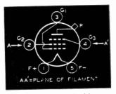
Tube Mounting Position VERTICAL—Base down. HORIZONTAL—Plane of filament vertical. C1=50  $\mu\mu$ f midget C2 C3 C4=0.005  $\mu$ f, mica C5 C8=0.002  $\mu$ f, mica, 5000 v. C6 C7=0.01  $\mu$ f, mica C9=1.5  $\mu\mu$ f/meter\* R1=8300 ohms, 4 watts L1=Tune to frequency "f" RFC=R-f choke T1=Filament transformer, 2000-v. insulation f=Operating frequency X=Insert keying relay here
