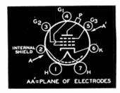
Tube Mounting Position VERTICAL or HORIZONTAL
