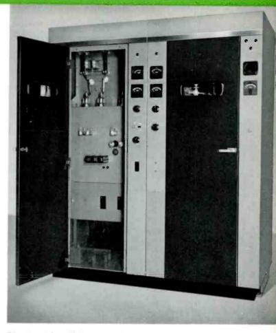
IPA and modulator driver stages of the BTA-ST can be seen at top of open cabinet. The exciter is at the center of the cabinet, and control equipment is placed just below the exciter.
