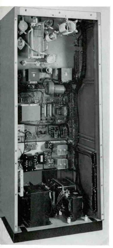
Rear view of BIA-1R1, with rear panels removed, showing vertical construction and accessibility of component parts.
