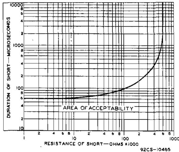
Fig. 3 - Thyatron-Type Shorts Test for Type 7587.
